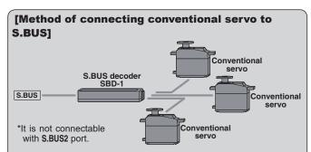
\* Items required: S.BUS receiver, SBD-1 S.BUS decoder, servo, SBC-1 channel changer or CIU-2 USB serial interface
