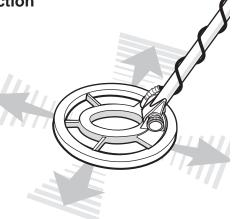
When pinpointing a target, try drawing an "X", as illustrated, over where the tone is induced.
