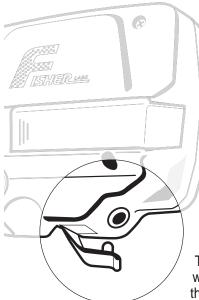
This detector has a 1/4" headphone jack. It works with any stereo headphone (not included) that has a 1/4" plug. When the headphone jack is connected, speaker volume is disabled. Using headphones extends battery life and prevents the sounds from bothering bystanders. Headphone use also facilitates detection of the weakest signals.
