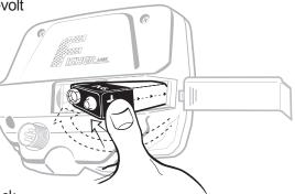
side of the Control Housing. Slide the battery door to the side to remove. Insert battery (see *illustration*). Close battery door. When it is time to replace the battery, simply pull up firmly on the end of the battery.
