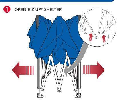
With a partner on the opposite side, grasp the bottom of the diamond-shaped area of **outer trusses** near the "OPEN HERE" sticker (see arrows for **outer trusses** on the diagram on page 11 for approximate location of "OPEN HERE" stickers).
