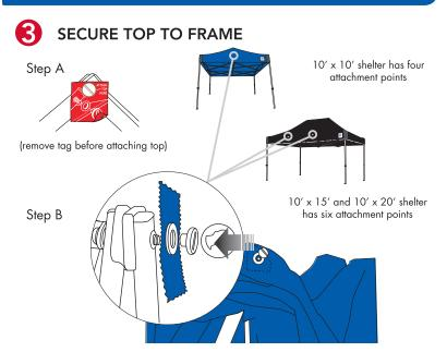
Line up the grommet holes on the sides of the fabric top to the frame top attachment points. The top attachment points on the frame are denoted by the RED tags.
