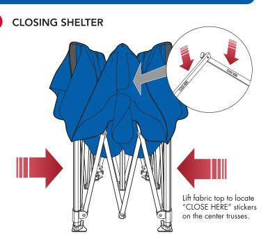
Grasp the frame on the top of the diamond-shaped area of center **outer trusses** on the opposite sides near the "CLOSE HERE" sticker.
