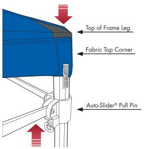
Fold up the fabric top corner to expose the Auto-Slider® Pull Pin.
