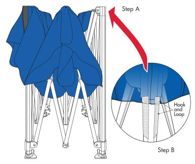
Gently unfold the fabric top, and place it over the semi-opened frame.
