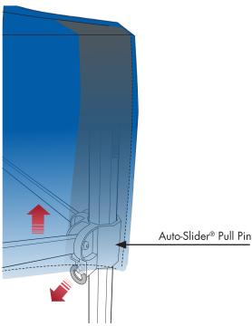
With one hand, slightly push up on the truss near the Auto-Slider® Pull Pin to relieve pressure.
