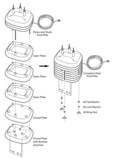
2. Place flat washers, lock washers, and plastic wing nuts over the protruding stud ends. Proceed to mount the shield. See "Mounting on Top of a Post:" on page 13.
