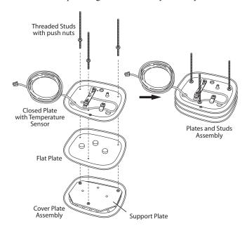
2. Place the plates and studs assembly aside and proceed to the appropriate instruction for your installation.
