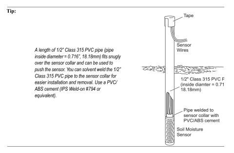
4. Carefully backfill the access hole with soil to eliminate any air pockets which could allow water to channel down to the sensor.
