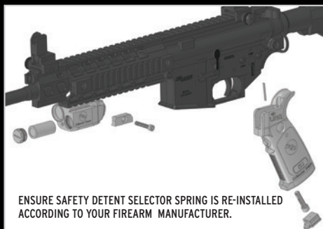
5. MOUNT GRIP TO FIREARM. TEST SAFETY SELECTOR TO ENSURE PROPER RE-INSTALLATION OF SPRING.
