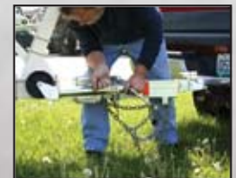
After the trailer weight has been applied to the hitch and the hitch is locked you may then unlock the Trailer Jack and raise into the "Out-Of-The-Way" position.
