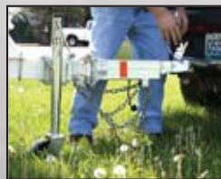
Crank counter close-wise to lower trailer into position.
