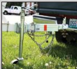
Roll trailer to position the hitch.
