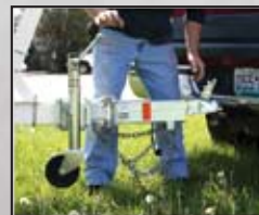
Lower trailer onto hitch after it is position. Continue to crank counter clockwise. Remember to lock to trailer onto the ball.
