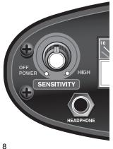
Sensitivity will be reduced slightly when using the Tracker IV in the Discrimination mode. If you want optimal depth capability, operate in the All Metal mode by turning the Discriminate control completely counterclockwise; then turn the Sensitivity control clockwise to its highest clockwise position without chatter. If your Tracker IV chatters or beeps erratically, reduce the Sensitivity by turning the left knob counterclockwise.
