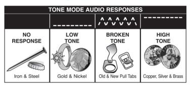
c. Adjust the DISCRIMINATION Control when encountering low-tone objects. If the Disc control can be adjusted to induce a broken (or scratchy) tone, the buried item is probably trash. A broken tone can usually be achieved between the 12:00 and 2:00 positions.
