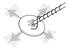
When pinpointing a target, try drawing an "X", as illustrated, over where the tone is induced.
