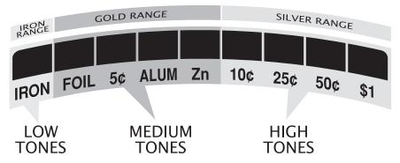
The faceplate label is color-coded above the Conductivity Arc. Ferrous, gold and silver targets will generally register within their corresponding color-coded ranges. Targets that are not gold or silver register within the same range according to their electrical conductivity.
