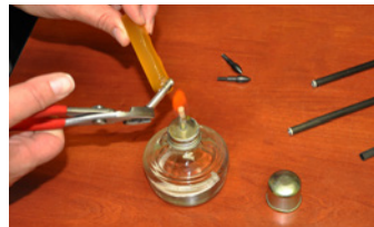
Heat the stick of adhesive with the flame until the adhesive glosses over
