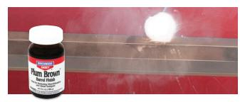
3 When the ideal temperature of 275°F has been obtained, apply Plum Brown Barrel Finish with a saturated swab in long even strokes. The rich plum brown color will appear immediately. (\*\*Fread Carmichel's Tip below).
