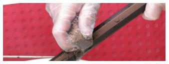
When browning is complete, rub all surfaces down with Barricade Rust Protection. This is very important after rinsing and will penetrate the surface and give you a deep, rich, mahogany-brown permanent coating. Allow to cure for 24 hours.
