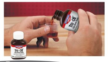
**2** First Finish Coat. Dip your finger into the cup and hand-apply Tru-Oil Gun Stock Finish in smooth, gliding coats. You'll find that this first coat will absorb readily into the grain. Be careful not to overcoat the first application, as this can cause unwanted build-up and possible runs (see picture on next page).
