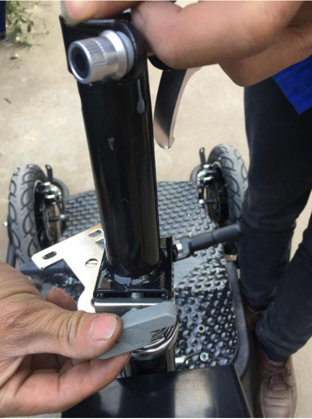
( 4 ) Install the pole, and screw the lock.
