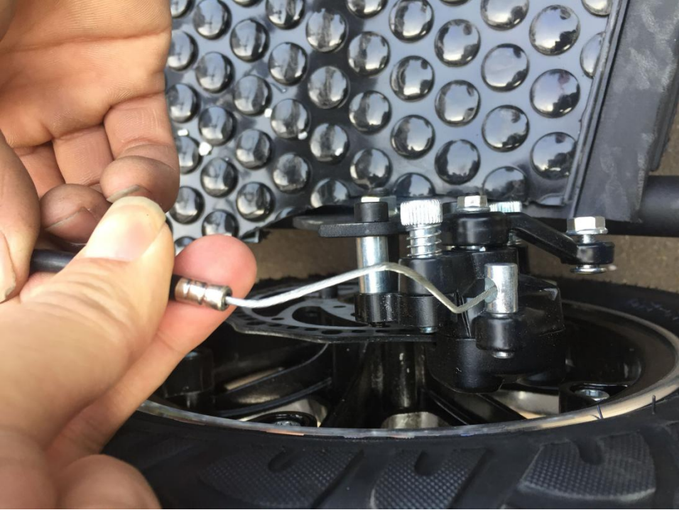
(2) Brake cable cross the hole of disc brake.
