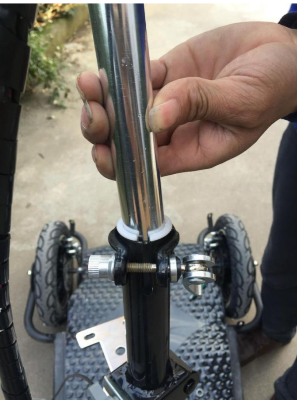
( 4 ) Install the pole, and screw the lock.
