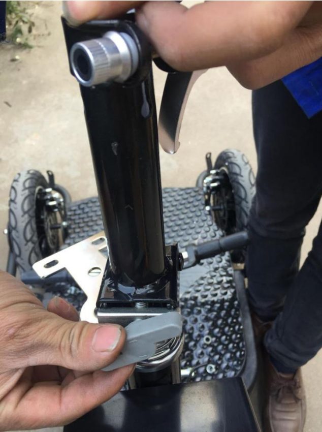
( 4 ) Install the pole, and screw the lock.
