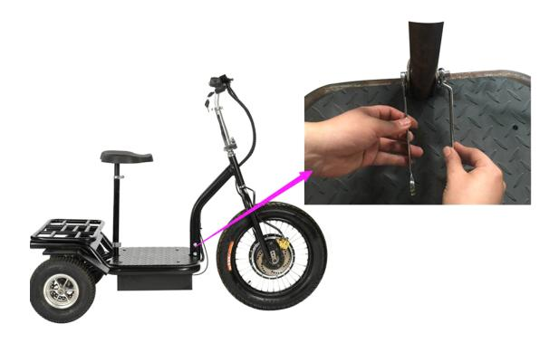
2. Handlebar. Inset handlebar and bolt, then screw it.
