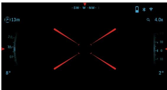
To measure the distance to a target using the laser rangefinder short press the POWER button. The rangefinder will take several measurements and will
