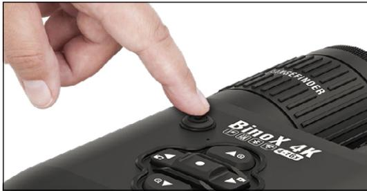
To TURN ON the device, press the POWER button.
