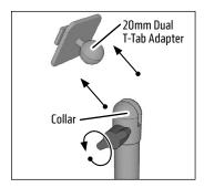
Depending on the size and weight of the tablet, either tablet holder may be connected to the Swivel Mount Adapter, but shouldn't be used for downward broadcasting. Use of the 25mm to Dual T-Tab Adapter is required. Note: the smaller 20mm to Dual T-Tab Adapter is not compatible with the shaft
