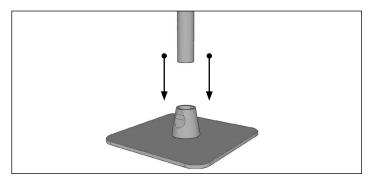
Connect the Dual Mount Assembly to the Dual T-Tab Pattern at top of Telescoping Shaft
