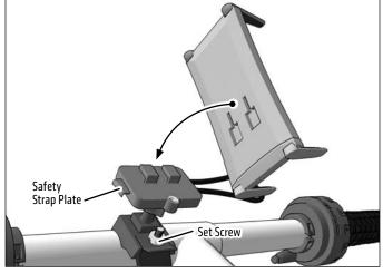
3 Remove mount by pulling up release tab and pushing strap back through slot.
