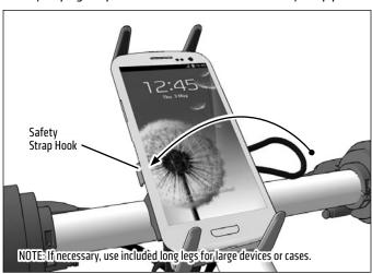
2 Attach safety strap plate to the 2T mount head and secure with set screw; attach holder to the safety strap plate.
