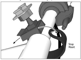
Insert device by pushing down on the lower support legs and engaging the spring-loaded mechanism. Secure with safety strap by looping strap across the device to hook on safety strap plate.
