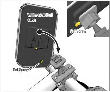
3 Insert device and adjust case position as desired, tighten adjustment ring to secure.
