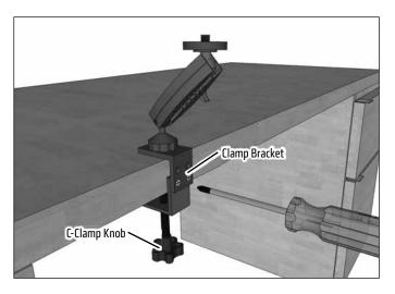
2 Loosen adjustment knob to adjust position. Retighten to set to desired angle.
