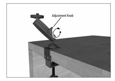
3 Attach camera (sold separately) with a standard 1/4"-20 socket to the screw on the mount head.
