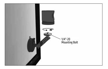
While pushing down on the pedestal, engage the suction lock lever to secure and attach pedestal to surface.
