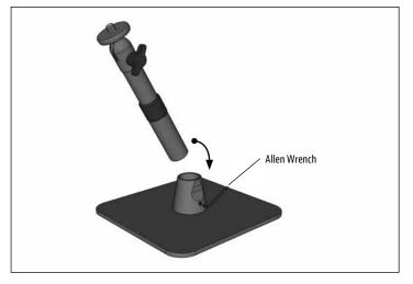
4 Adjust the height and angle of the mount by loosening the adjustment ring and the adjustment knob. Retighten to set.
