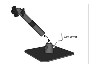
2 Attach any Arkon Dual-T holder (sold separately) to the pedestal by inserting the Dual T-Tabs into the holder's Dual T-Slots and pushing down to lock.
