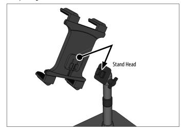
3 Adjust the height and angle of the mount by loosening the adjustment ring and the adjustment knob. Retighten to set.
