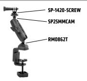
Attach pedestal clamp by turning the c-clamp knob; adjust the clamp bracket position if necessary with a Phillips screwdriver. To attach the camera head adapter, loosen the adjustment knob, insert the adapter, and retighten to desired position.
