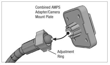
Remove quick-release attachment from camera mount plate and attach to camera.
