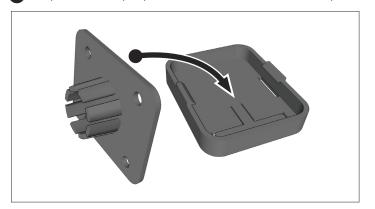
3 Snap the combined AMPS adapter/camera mount plate onto the mount head then re-tighten adjustment ring.
