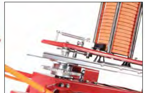
Throwing arm is gear-driven for smooth, reliable operation
