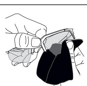
2. Once the inside lens mounting tab is free, continue pivoting the lens until the mounting tab on the end of the lens easily releases from the frame.
