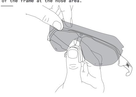
2. Gently apply pressure on the lens with your thumbs while applying slight pressure in the opposite direction with your finger on the frame. This will cause the remaining lens mounting tab to « pop » into place in the frame.
