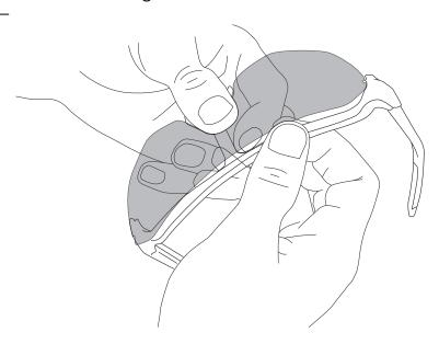
3. Once the lens is free from the top of the frame, it will easily release from the nose piece.
