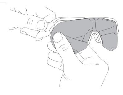
2. Hold the top frame in the center of the glasses with one hand while grasping the center of the lens near the nose area with the other hand. Gently pull apart to release the mounting tab from the frame.
