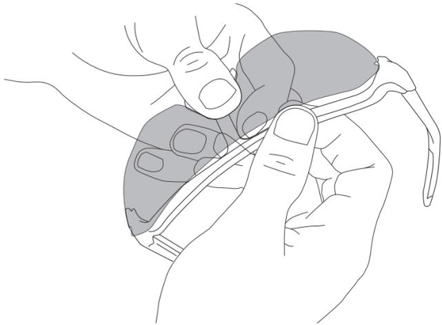
3. Once the lens is free from the top of the frame, it will easily release from the nose piece.
