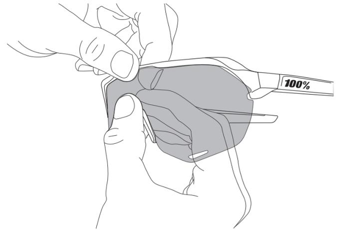
3. Gently insert the lens into one end by inserting the mounting tab into the frame. Repeat on the other end.
