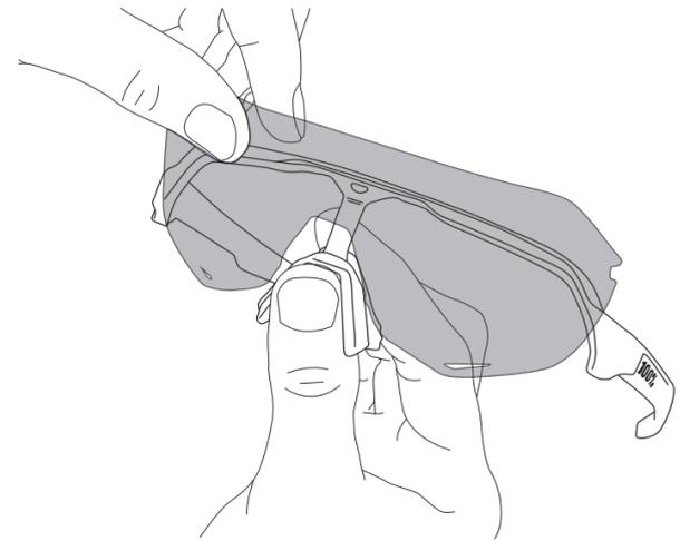
2. Gently apply pressure on the lens with your thumbs while applying slight pressure in the opposite direction with your finger on the frame. This will cause the remaining lens mounting tab to « pop » into place in the frame.
