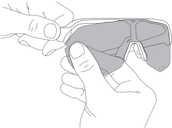
2. Hold the top frame in the center of the glasses with one hand while grasping the center of the lens near the nose area with the other hand. Gently pull apart to release the mounting tab from the frame.
