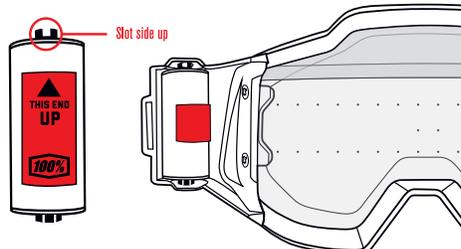
4. Remove one side of the red tape from the film roll such that the film can unwind with the tape still attached. The sticky side of the tape should be facing you.
