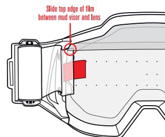
6. Begin pulling the film across the lens, towards the right. Hold the film roll with one hand to keep the roll tight.
